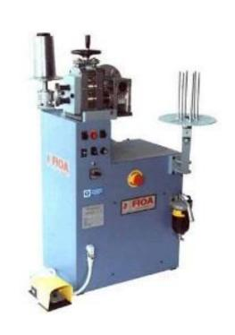
MOTORISED WINDER FOR WIRES AND TUBES COMPLETE WITH
