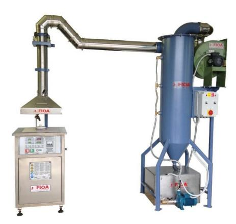
COMPACT PICKLING UNIT FOR INGOTS COMPLETE WITH HEATER, RINSING TANK AND SUCTION FAN.
