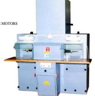
DRY BARRELING UNIT COMPLETE WITH - WOODEN ROTATING OCTAGONAL DRUM.
